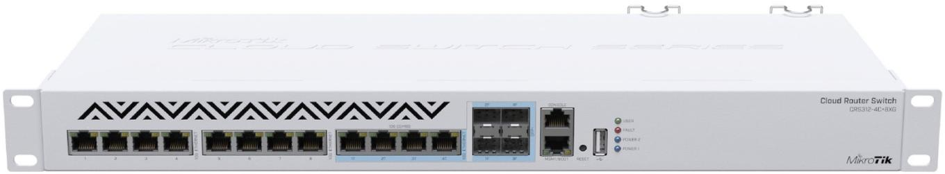
CRS312-4C+8XG is 8-port Gigabit Ethernet switch with four 10g Ethernet / SFP+, combo ports. Includes all basic functionality for a managed switch and more.
